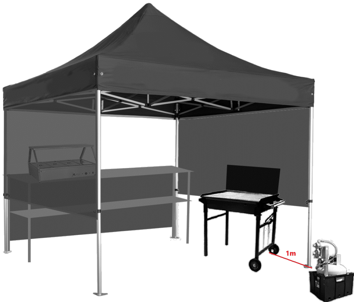
Figure 12: Adequately ventilated stall setup. Keep the regulator vent away from source of ignition by at least 1m
